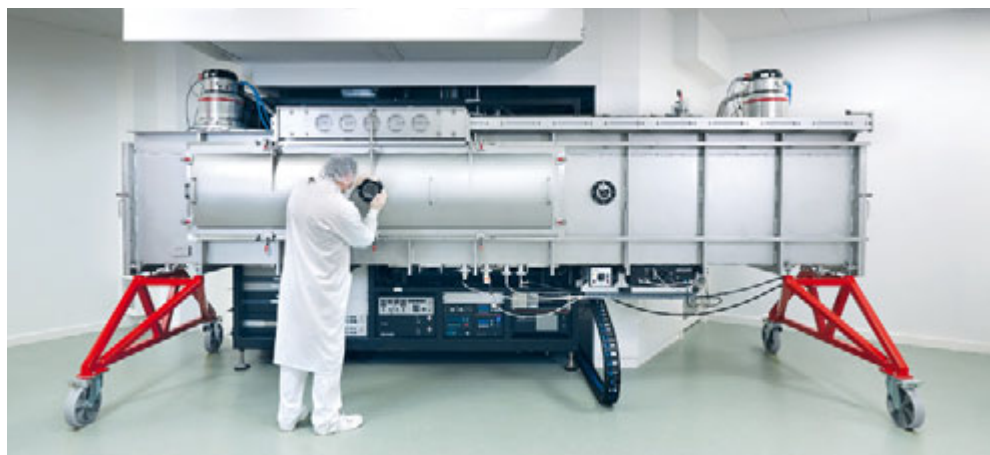
"Maxima", the patented IBS coating machine for large optics (long shapes)
