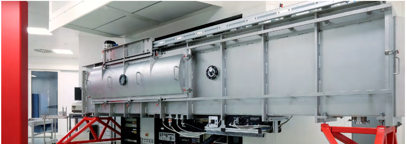
"Maxima", the patented IBS coating machine for large, rectangular optics
