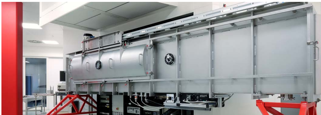
"Maxima", the patented IBS coating machine for large, rectangular optics
