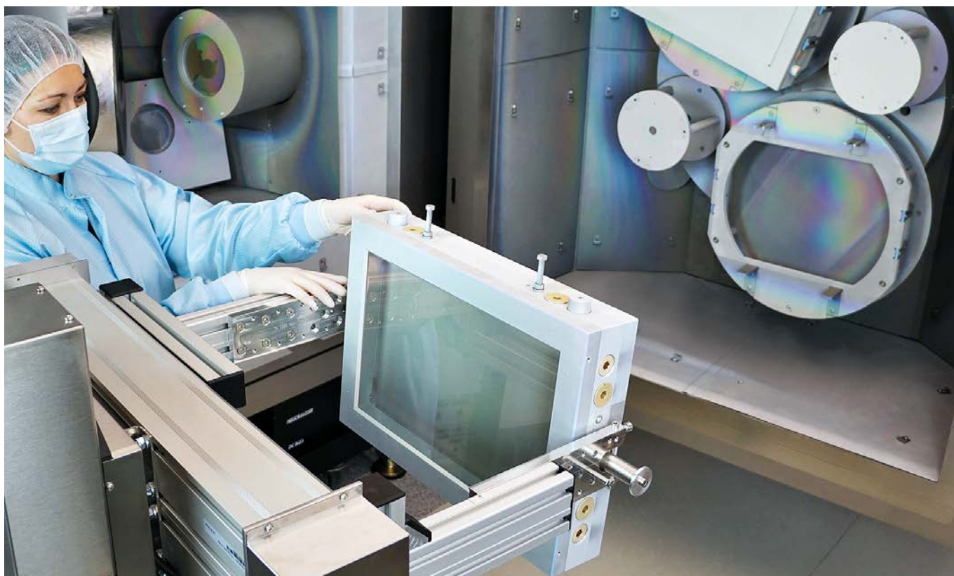
"Teresa", the largest IBS machine, suitable for substrates up to Ø 550 mm
